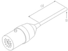
ends. This can be achieved by supporting the cable with ties at points 's' shown in the diagrams. Distance 'd' should be between 20 and 50cm. The cable should be slack between the tie and the connector. In bakeout zones stainless-steel cable ties should be used.
