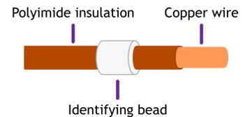
Polyimide is strong, flexible and abrasion-resistant and therefore difficult to strip. The simplest method of stripping polyimide film is to cut a ring with a sharp knife and withdraw the cylinder of insulation over the end of the wire.
