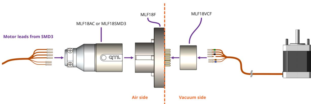
**i INFORMATION:** Verify that the motor is working correctly before sealing the vacuum chamber. Rectifying mistakes afterwards is inconvenient.
