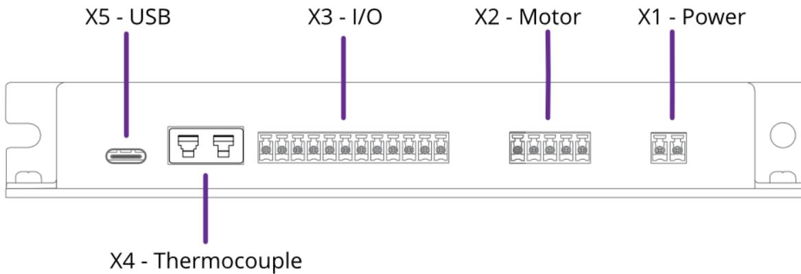
The Power, Motor and I/O sockets use 3.5 mm pitch pluggable rewireable terminal blocks. These are suitable for 28 – 16 AWG (1.5 mm<sup>2</sup> max.) stranded wire. Strip insulation to approx. 6 – 7 mm before securing the wire in the terminal block.
