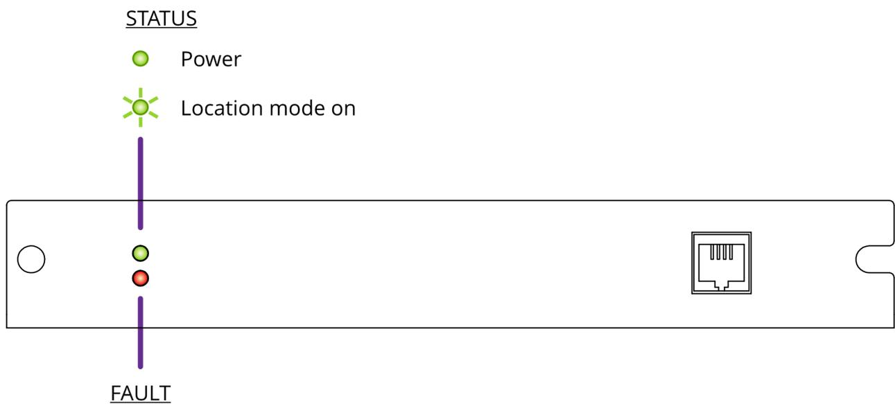
The fault indicator flashes or remains lit if the SMD3 is in a fault state (see section [Faults](#) for fault indications). When a fault is present, motor operation is disabled.
