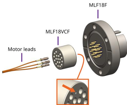
Alternatively, plug crimps directly onto the feedthrough pins of the MLF18F:
