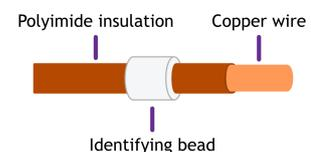
Polyimide is strong, flexible and abrasion-resistant and therefore difficult to strip. The simplest method of stripping polyimide film is to cut a ring with a sharp knife and withdraw the cylinder of insulation over the end of the wire.
