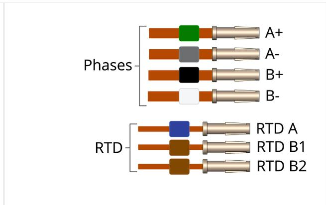
If the identification beads have been removed, the wires can be identified using an inexpensive multimeter, and a magnet. The multimeter must be capable of measuring resistance with a resolution of about 1 ohm.
