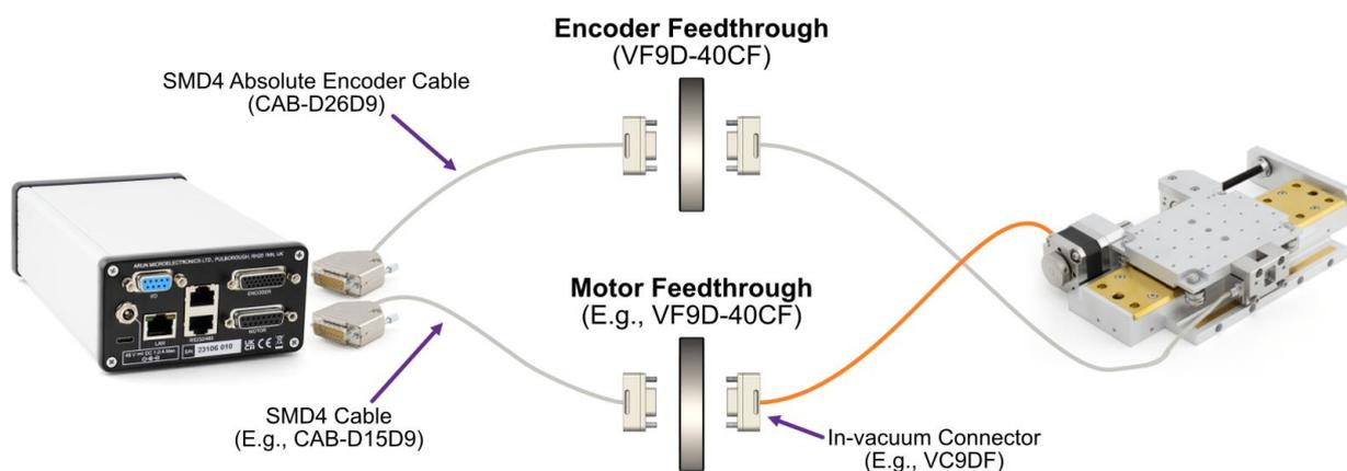
Absolute scales are patterned in such a way that the readhead can determine without any prior reference exactly where it is positioned, much like looking at a ruler. The absolute encoder therefore knows its absolute position at any time. The electronics can be powered off, the mechanism moved, and powered back on, and the readhead can still determine its absolute position.
