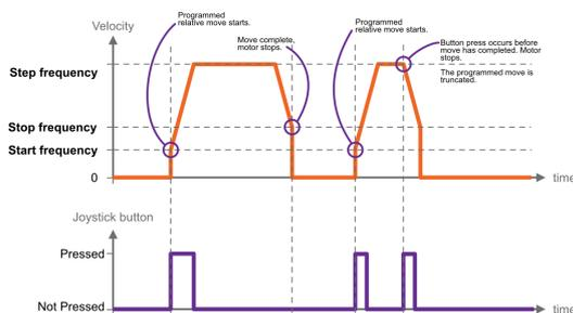
Trigger a pre-defined relative move with the joystick.
