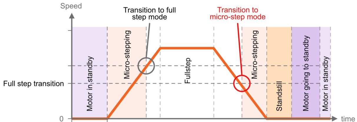
The resolution to use during microstepping is configurable, via the microstep resolution setting [RES]. Choices are 8, 16, 32, 64, 128 and 256. In all modes except for step/direction, the motor is only stopped in full-step positions. Microstepping is used exclusively for the purpose of smoothing the transition between steps, not to increase resolution.
