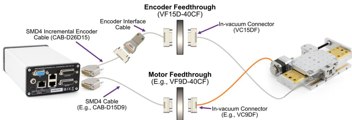
The position is volatile and stored only in the counter on the SMD4, unlike in the case of the absolute encoder. The incremental encoder only provides pulses which are used to increment or decrement a
