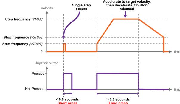
A short button press (< 0.5 s) causes a single step in the commanded direction. This is useful for precise positioning.
