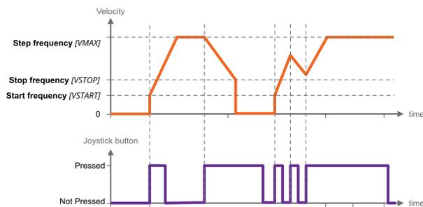
Motor accelerates toward target frequency on joystick key down. Continuing to hold the key down has no further effect.
